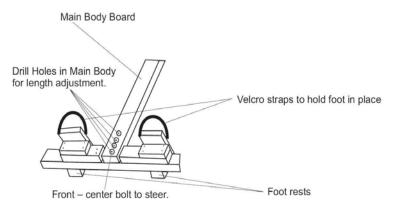
Put a washer between axle frame and main body board
